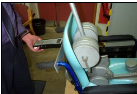
Figure 3: Measurement of push effort
