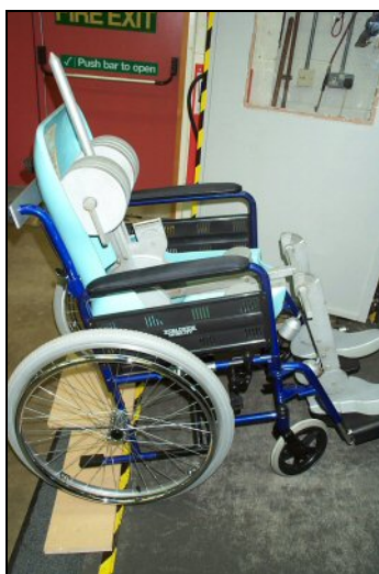
Figure 2: Wheelchair and manikin used in test measurements
